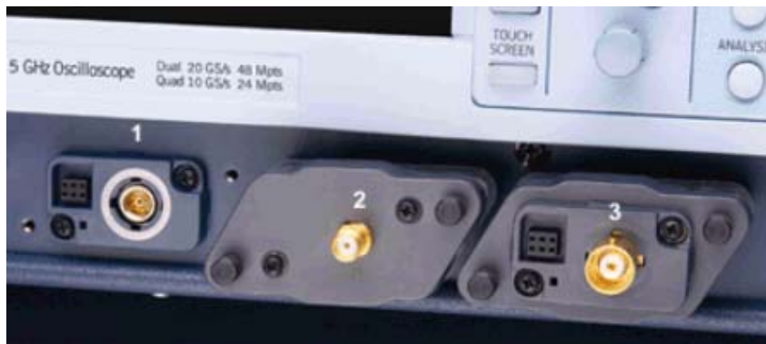
(1) BMA Female Connector, (2) ProLink BMA-to-SMA Adapter Installed, (3) ProLink BMA-to-BNC Adapter Installed
