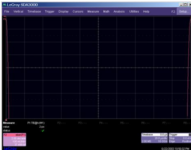
Figure 10. The bathtub curve is constructed by rescaling the total jitter curve in Figure 9 to one unit interval, and centering the right side of the total jitter curve at 0 UI and the left side at 1 UI (the left
